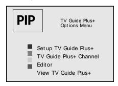
☐ "Setup TV Guide Plus+" is where you will set up TV Guide Plus+ to control your TV. The information for this procedure is on pages 18 to 22.
